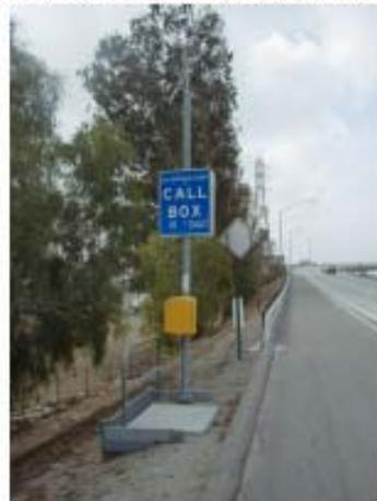
"F" site is placed behind a guard rail or another barrier and faces perpendicular to the road.
